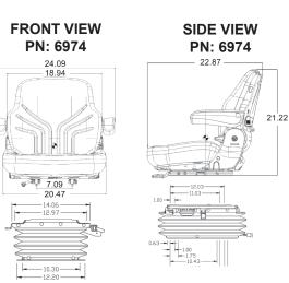
\*Drawings show seat top without backrest extension and seat depth/tilt adjustment handles.
