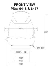
\*Drawings show mechanical suspension only and do not show swivel.
