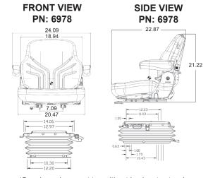
\*Drawings show seat top without backrest extension and seat depth/tilt adjustment handles.
