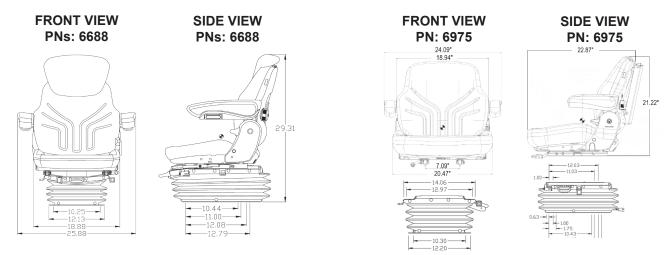
\*Drawings show seat top without backrest extension and seat depth/tilt adjustment handles.
