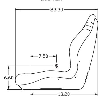
Drawings shown do not include measurement of the hinge bracket.
