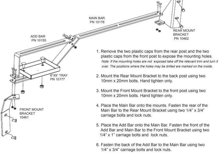
7. Mount the Tray to the Main Bar at desired location using two 1/2" x 1" carriage bolts and lock nuts.
