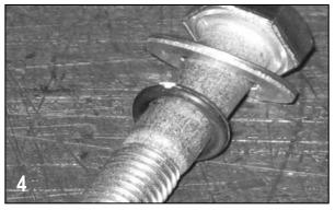
Clean the threads of the bracket screws (12715A) thoroughly. Once clean, install the four flat washers (12901) and four screw head O-rings (12717) onto each of the bracket screws.
