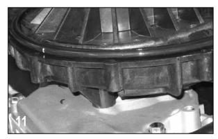
Place the pump body O-ring (12719A) around the outside flange of the rear bracket. The O-ring may be sparingly lubricated with silicone to ease installation of the pump body in the next step.
