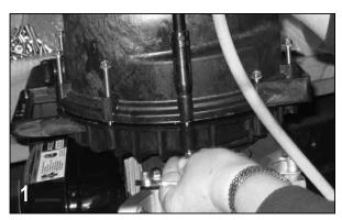
Remove the 10 body screws (12720), lock washers (V07018) and nuts (V07019) from the pump assembly. Remove the body from the pump assembly.
