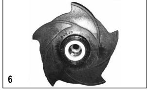
Verify impeller hex nut (12775A) is located at the bottom of impeller snout (should be installed). A very light press fit may be required to install nut into cavity. Install the ceramic seal half into hub of impeller by using an arbor press or similar tool. Outside diameter of rubber boot may be sparingly coated with silicone to ease installation.
