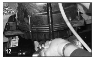
Install the pump body (12712/13712) as shown below with the outlet flange facing up. Install the 10 body screws (12720), 10 lock washers (V07018), and 10 nuts (V07019) to secure the pump body to the rear bracket. Tighten the bolts securely all the way around.
