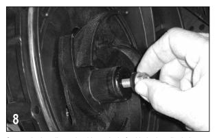
Secure the impeller to the drive unit shaft with the impeller bolt gasket (12774VA) and impeller bolt (12765A). Tighten the impeller bolt until snug.
