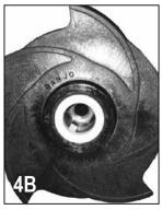
4A: Screw the supplied 7/16-14 hex head cap screw into the impeller snout. As the bolt is tightened the impeller will be pried off of the shaft of the drive unit. Remove the 7/16-14 screw once the impeller has been removed from the drive unit. 4B: If the pump impeller is going to be reused the ceramic seal half (12713) should be removed from the impeller at this time. The impeller key (12902A) located behind the ceramic seal half should be replaced at this time
