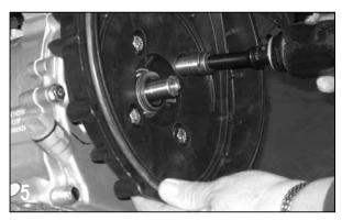
Install the rear bracket onto the drive unit using the bracket screw assemblies from the previous step. The handle of the rear bracket should be to the top of the drive unit. Tighten the screws securely.
