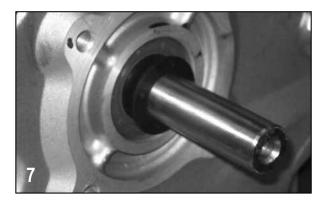
At this time, it may be necessary to polish the drive unit shaft to remove any corrosion that may have formed.
