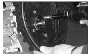
Remove the four bracket screws (12715A), rear bracket washers (12901), and screw head O-rings (12717) from the rear bracket using a 1/2" socket. With the four bracket screws removed, the rear bracket can now be removed from the drive unit.
