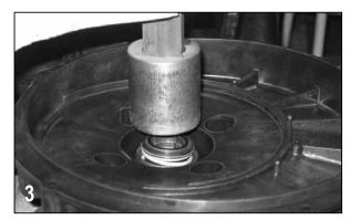
To install the carbon seal (12713) half into the rear bracket use a tool such as a 1 ½" pipe nipple or arbor press to give even pressure on the metal flange of the seal housing during installation. Gently press the seal into position until it bottoms.
