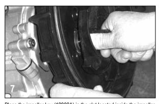
Place the impeller key (12902A) in the slot located inside the impeller snout. The impeller (12771A/12772/13772) is now ready to be slid onto the drive unit shaft.
