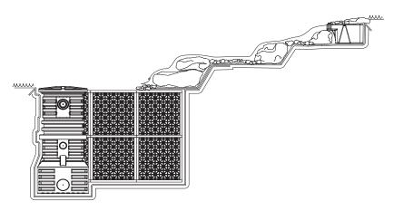
Once excavation is complete, install underlayment, pond liner, properly oriented Eco-Blox and Pump Vault. Backfill the space between the Eco-Blox/ Pump Vault and the excavation to lock them into place, either outside the liner with sand or clean fill, or inside the liner with gravel 3/4" or larger in diameter. Top the liner and basin with 3/4" or larger gravel or decorative stone.
