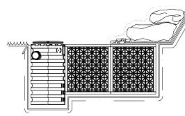
The PV1700 flat panel will sit flush against the Eco-Blox, so that water can enter the pump vault. The area where the pump vault will sit should be dug 22" deep for the PV1700. When using Eco-Blox, the pump vault will recess lower than the Eco-Blox. The area for the Eco-Blox to sit should be dug 18" deep.
