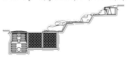
For installations where a larger basin volume or deeper basin is required, Atlantic offers pump vault extensions for both the PV1800 and PV2300. Each extension will add the height of one Eco-Blox. For each additional Eco-Blox layer, increase the depth of your excavation by 17".
