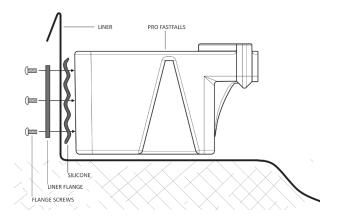
Apply Atlantic's Silicone Sealant in a continuous, consistent bead along the center of the threaded inserts. Once completed, return the liner to its dry-fit position.
