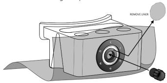
Tighten flange screws with a hand held screwdriver only. Over tightening the screws could strip out the inserts or crack the liner flange. The screws need only to be snug for the silicone to make a seal.
