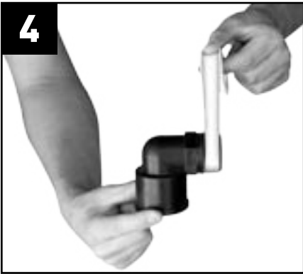
4 Put teflon tape onto 90° elbow.
