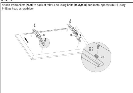
Attach TV brackets (N,M) to back of television using bolts (M-C, M-D, M-E) and metal spacers (M-F) using Phillips head screwdriver. If bolts are too long, spacers (M-G, M-H) may be required.
