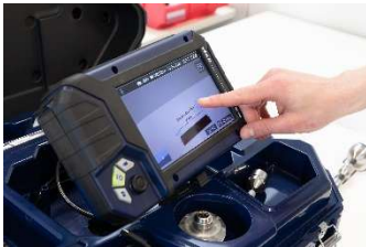
Fig. 53: Set the start and end point of the measuring segment.
