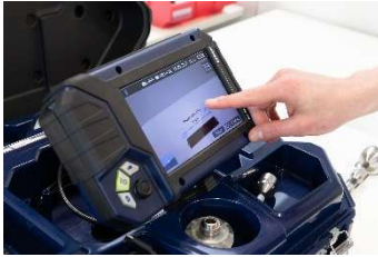
Fig. 48: The measuring points can be moved by dragging them
