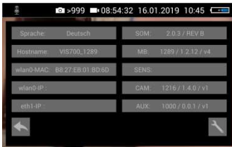
Fig. 55: Info menu with SOM (Firmware of the camera) and CAM (Version of the camera head)
