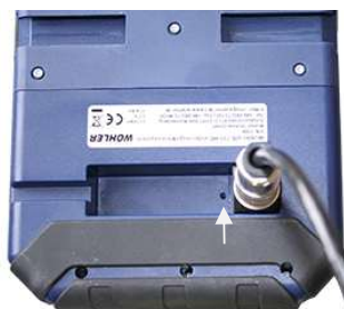
Fig. 70: Reset hole indicated by an arrow
