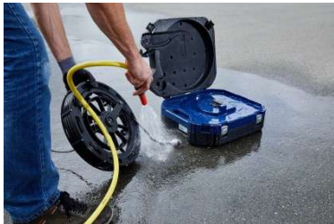
Fig. 78: Cleaning the viper and the rod
