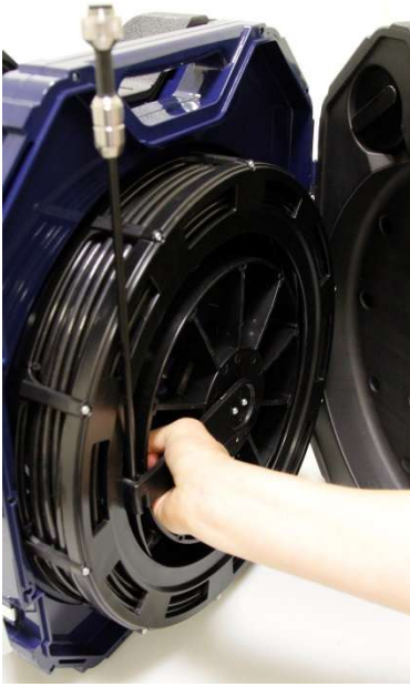
Fig. 75: Grasping the end of the rod and the viper
