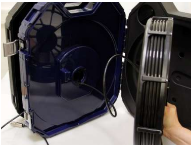
Fig. 76: Removing the viper with the connection cable from the case.
