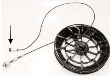
Fig. 77: Viper removed from the case, monitor plug covered by a lid
