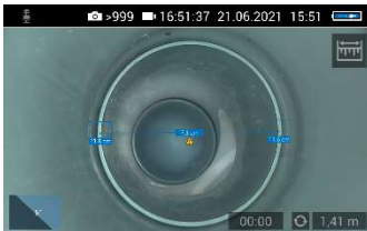
Fig. 47: Warning triangle under distance indicator
