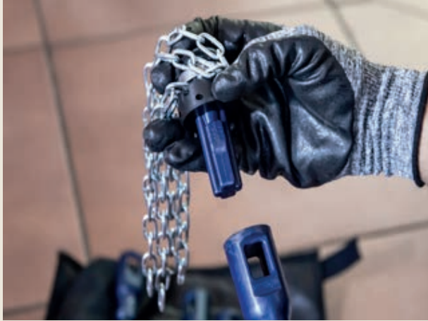
You can attach the cleaning attachment to the rod with just one click.
