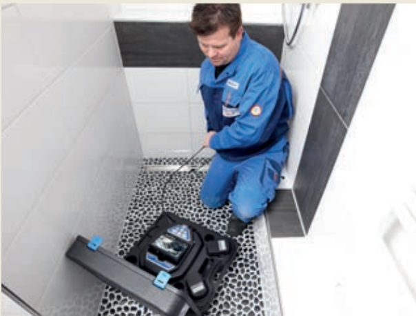
This camera head with a diameter of 1" is tough and can withstand water pressure up to 3 bar. It's perfect for navigating through pipes that are 1.5" in diameter, even if they have multiple bends of up to 87°.
