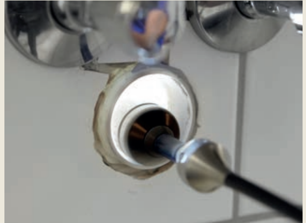
The color camera head produces crystal-clear images, even in dimly lit areas, thanks to its 12 LEDs.
